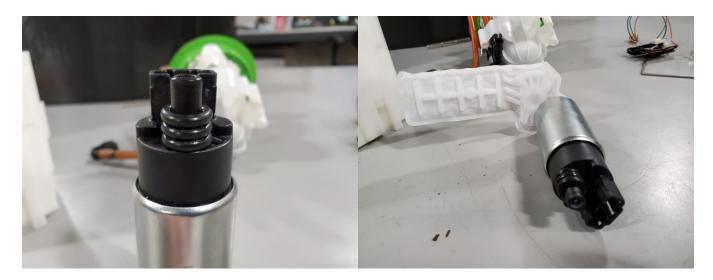
8 – Install the pump into the center section, seating two of the O-rings all the way into the module, the 3<sup>rd</sup> O-ring acts as a spacer to prevent the other two from pushing down with fuel pressure.
